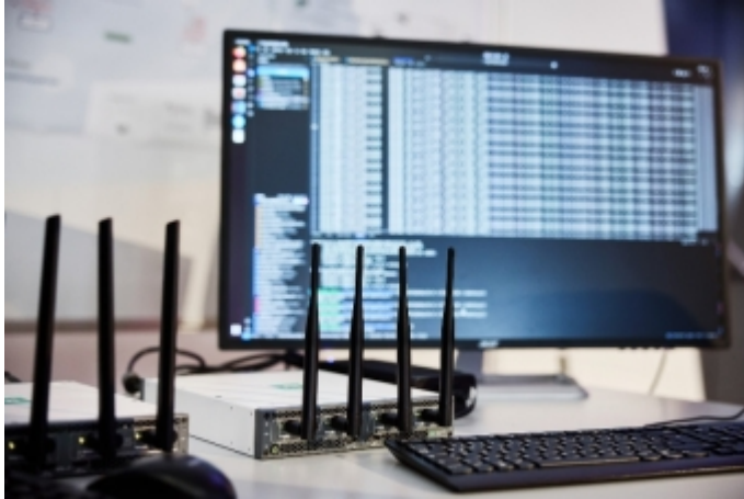
The software-defined radio demonstrator by LUH is able to work in the 3.8 to 4.2 GHz range
